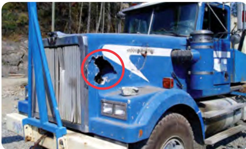
Fly rock thrown from a poorly controlled blast damages a vehicle.
