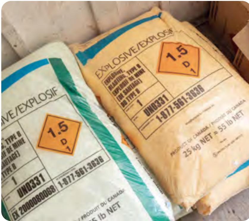
Blasting agents are either dry (free-running) or slurry products. Most dry types of ANFO mixtures have no water resistance, so a plastic *liner* (sock) may be required for wet holes. Dry products are generally supplied in bulk or packaged in bags with oil- and water-resistant liners. When free-pouring ANFO, follow the manufacturer's recommendations for the minimum diameter of the drill hole. These will vary between suppliers.
