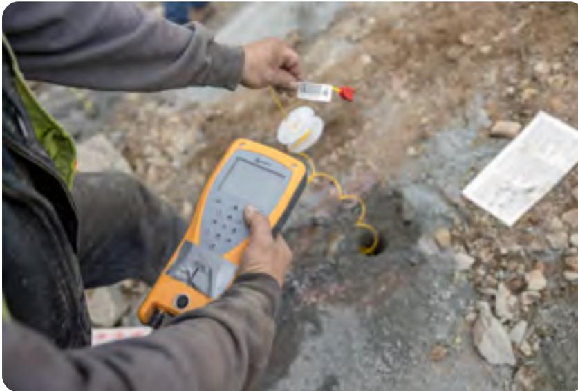
A worker uses a bench tester to communicate with a wired electronic detonator.
