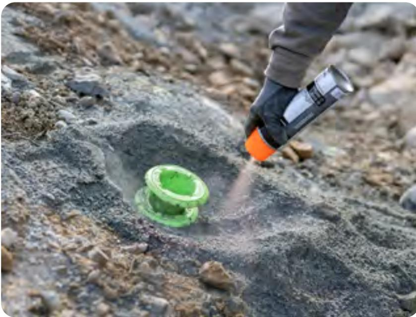
Marking an anomalous hole with double cones and spray paint
