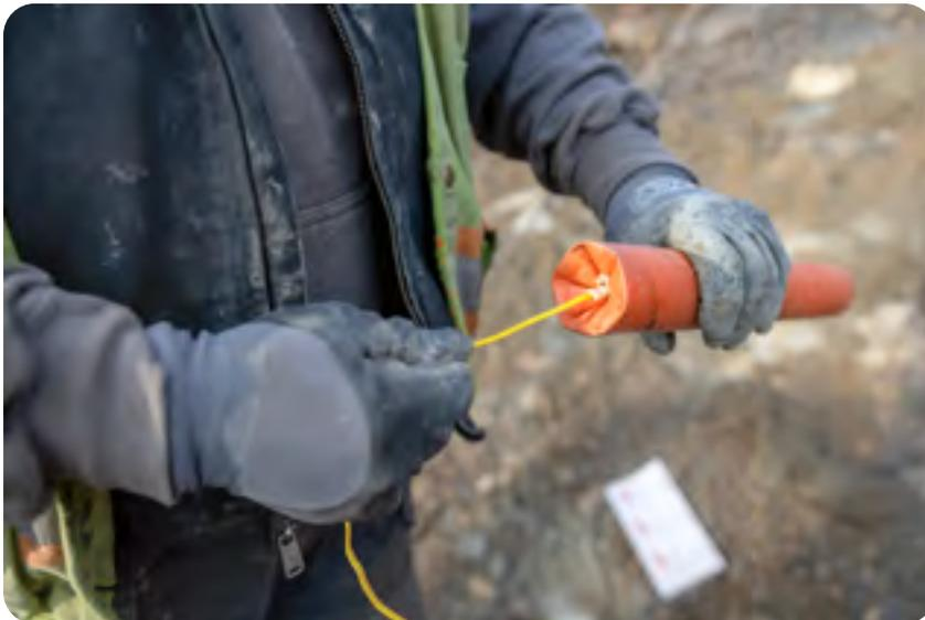
A worker prepares a primer. The detonator is already inserted in the stick of dynamite.
