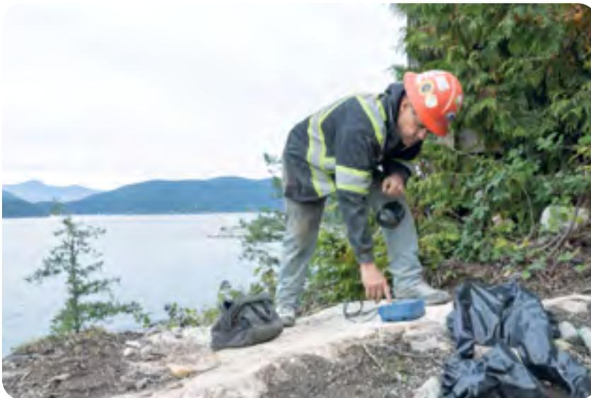
A worker uses a seismograph to measure ground vibration.
