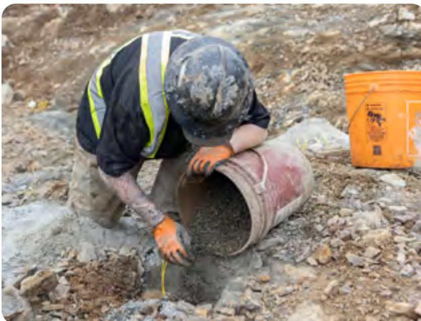
A worker carefully pours stemming into the collar of a blast hole.
