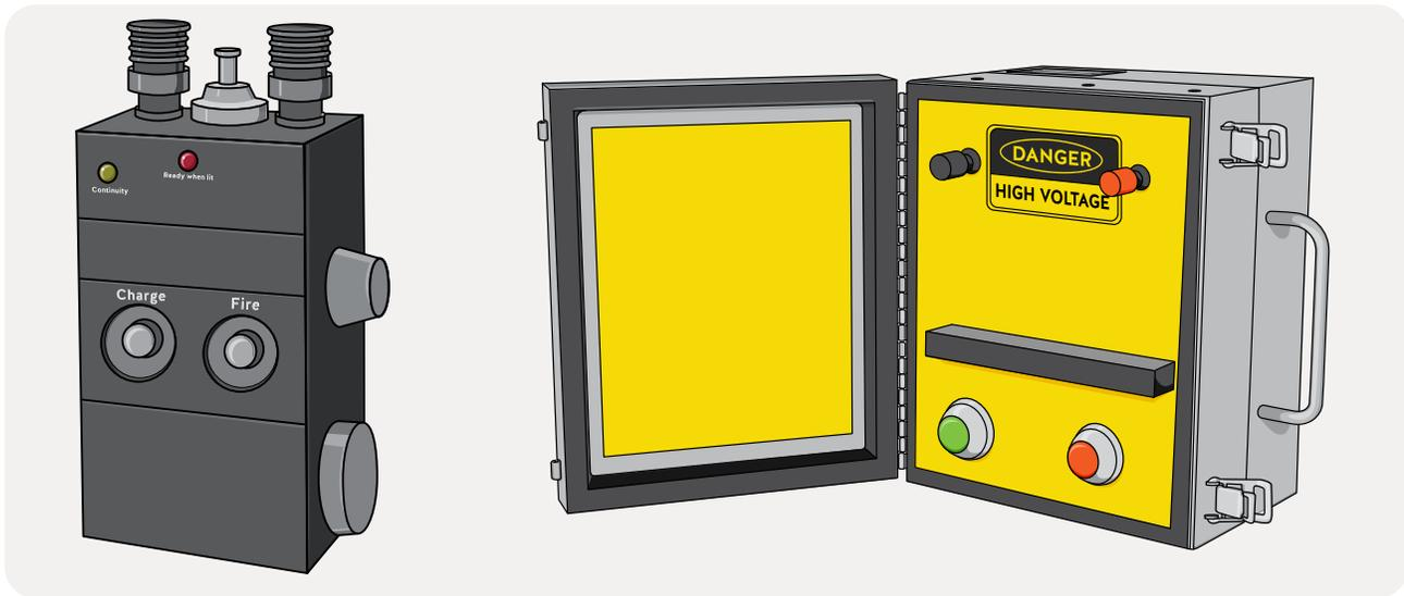
At left, a 50-shot blasting machine — an example of a capacitor discharge machine used to fire a single series circuit. At right, a 200-shot condenser — an example of a capacitor discharge machine used to fire a multiple series circuit.
