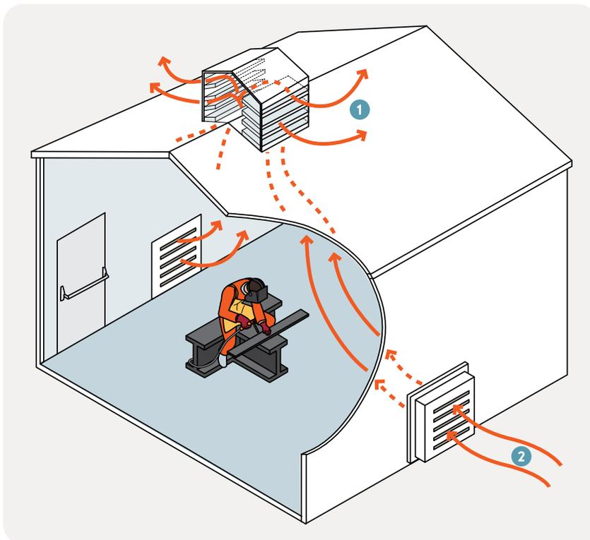
Dilution ventilation is an additional control that helps prevent buildup of welding fumes and protects workers in adjacent areas.
