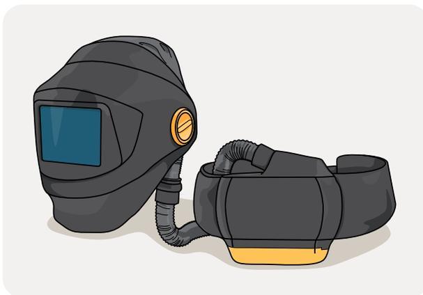
PAPRs are available with an integrated welding visor to protect the skin and eyes from UV and to provide a clear viewing window. This device allows a welder to keep the respirator in place when checking a weld. If a welder has to lift the visor to check a weld, they should wait until visible fumes have disappeared before doing so.
