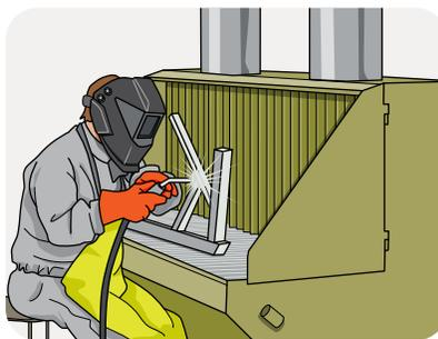
Extracted workbenches are ideal for workpieces that can be transported to the workshop.
