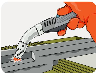
On-torch capturing hoods are useful when welding larger workpieces that are too big to transport to a workbench.
