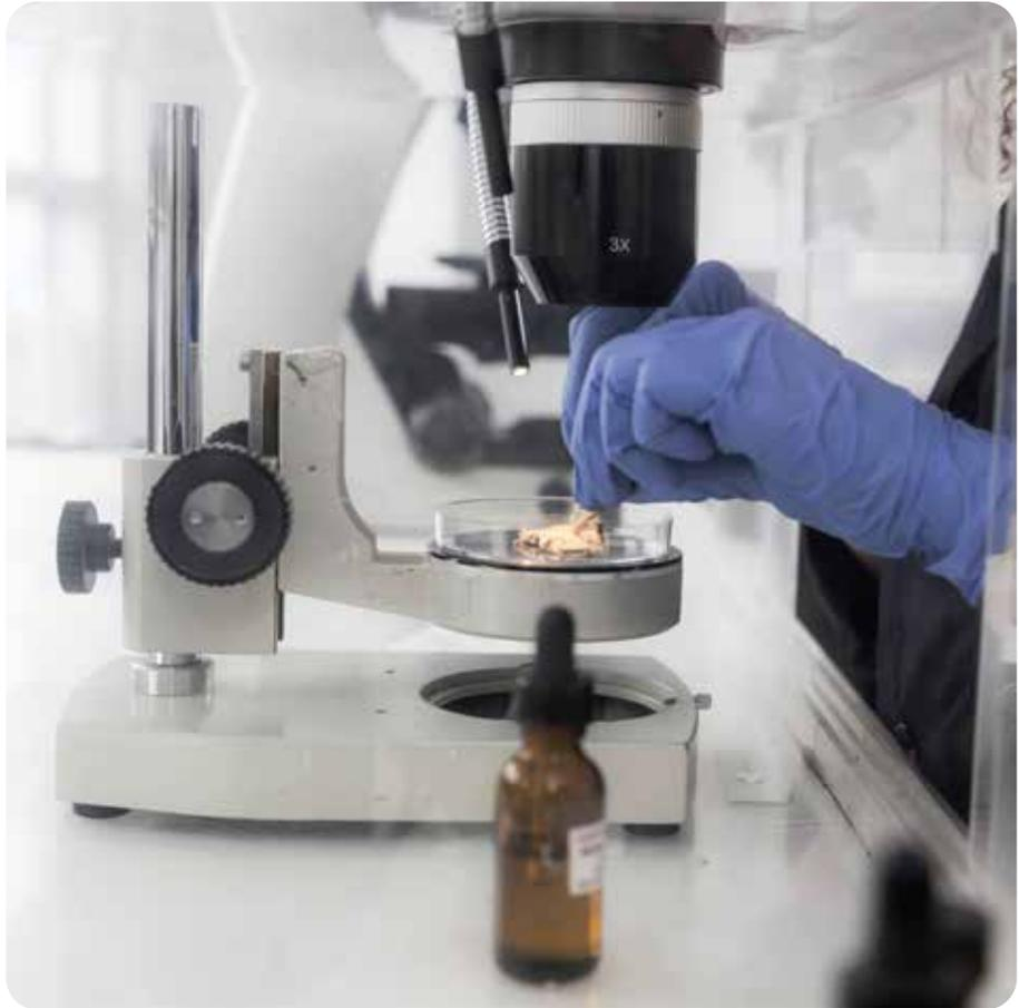
Figure 3: Analyst preparing a sample for asbestos identification.
