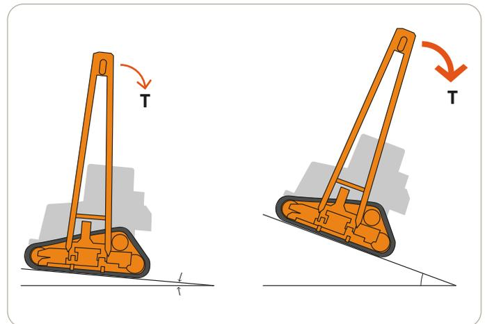
At left, a side-boom pipelayer on a slope. Lowering the boom angle and increasing overhang reduces fore-aft torque.
