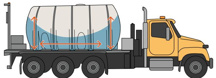
The arrows indicate how the weight of a live load and its centre of gravity can shift. Liquid sloshing around in the tank can have a significant effect on the vehicle's handling and stability.
