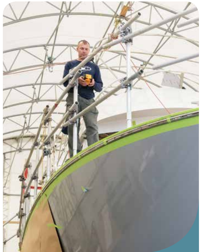
Coastal Craft fitter Tamas Mihalyi is protected by the guardrails as he installs the ship's deck lights.
